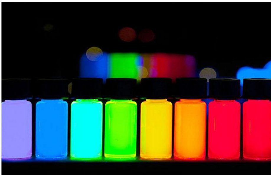
Alexei Antipov, Quantum Dots with emission maxima in a 10-nm step are being produced at PlasmaChem in a kg scale (CC BY-SA 3.0 via Wikimedia Commons)
